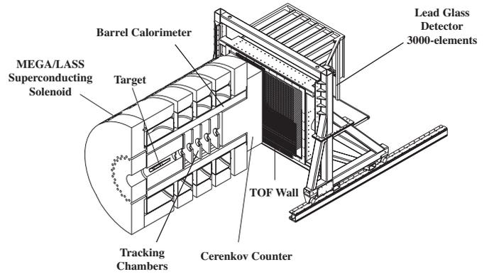
**Fig. 2.** Schematic view of the detector in Hall D
