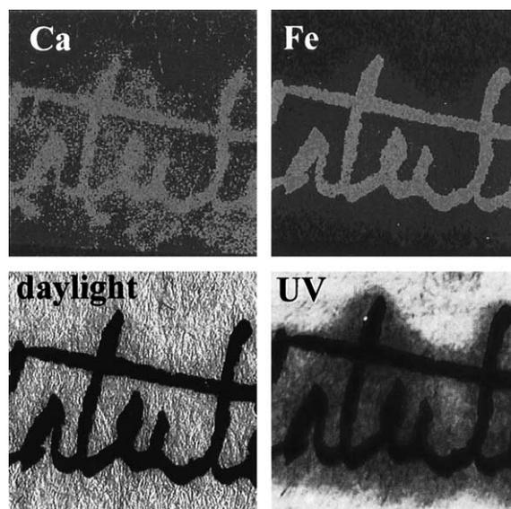
Fig. 3. Elemental maps and visual aspects under daylight and UV light of an altered manuscript showing the migration of Ca and Fe around the characters written using an iron-gall ink. The scanned area is  $10 \times 10 \text{ mm}^2$ .
