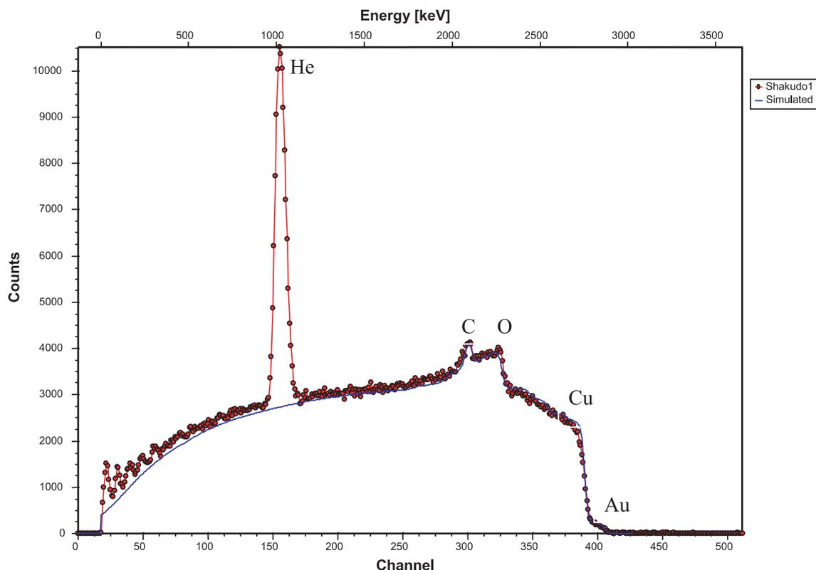
Fig. 4. RBS spectrum of the hilt of a historical Japanese sword. The hilt is made of a traditional Au/Cu alloy named *Shakudo* covered with a patina composed mainly of copper oxide and a varnish layer. The spectrum is obtained with an external 3-MeV proton beam in a helium atmosphere, producing an intense He peak which can be used for dose monitoring and energy calibration.
