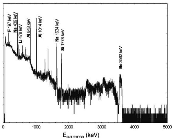
Fig. 2. PIXE and PIGE spectra of ancient emerald set on Visigoth royal crowns excavated in Guarrazar, Iberic Peninsula (8th century A.D.). In addition to the main constituents of the emerald (Be, Al, Si), the two PIXE and the PIGE spectra show various trace elements (Li, F, Na, Mg, Ca, Ti, Rb, Ni, Cu, Zn, Cs) used to infer the origin of these gemstones.
