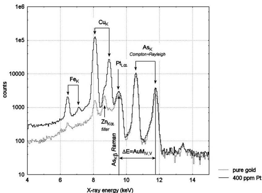
Fig. 6. PIXE-XRF spectra recorded on pure gold and a gold sample containing 400 ppm platinum. The peak rising at 9.4 keV corresponds to the overlap of the Pt signal and the Raman scattering of the As  $K\beta$ . Using this setup, the detection limit of platinum was lowered to 50 ppm, compared to 1000 ppm at best for PIXE.
