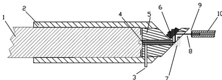
Fig. 5. PIXE-XRF layout for the in-air measurement of platinum in gold. (1) Housing of the Peltier-cooled *silicon-drift* detector for the collection of fluorescent X-rays. (2) Setup housing. (3) Helium inlet for cooling the intermediate As target. (4) Zinc absorber in front of the Si crystal. (5) Aluminium part. (6) Arsenic intermediate target. (7) Gold sample being analysed. (8) Proton beam. (9) Exit window. (10) Beam line.
