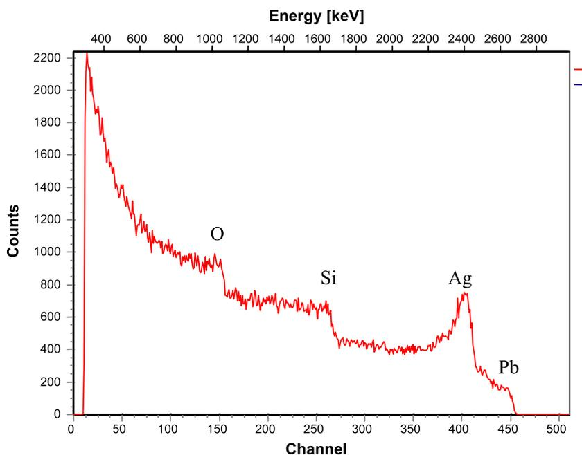
Fig. 7. RBS spectrum of a fragment of a lustred Islamic ceramic obtained with 3-MeV alpha external beam. The lustre is a lead-rich glassy layer containing silver aggregates.
